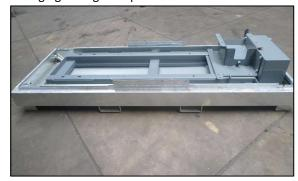
The drip tray has a capacity of 270 l, which is larger than the contents of the fuel tank and oil pan combined.
