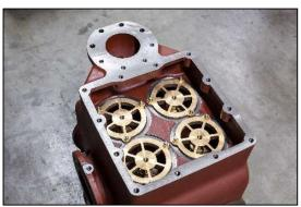
Bronze valve seats and optimal hydraulics ensure the highest efficiency and the best vacuum.
