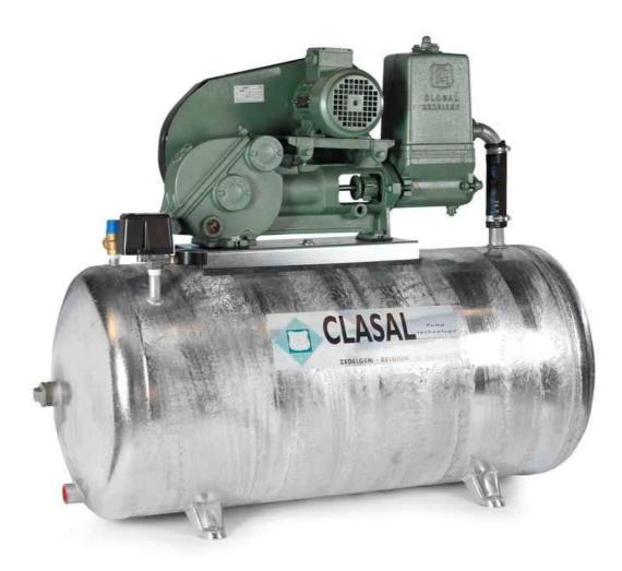
Piston pumps in combination with a horizontal or vertical water pressure reservoir form a hydrophore group. There is an air cushion in the reservoir. The pressure switch allows the pump to be switched on and off.
